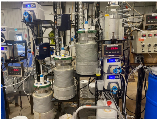
Magnesium Hydroxide Pptn (3 reactors)
