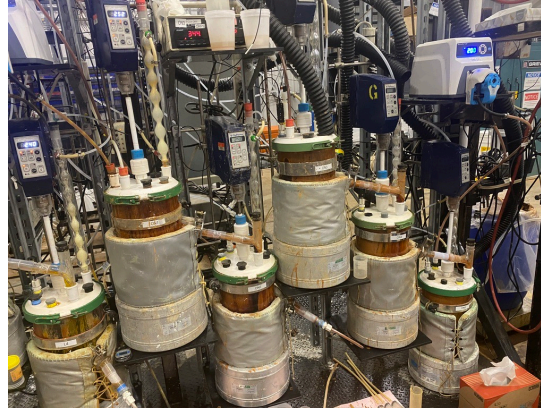
Olivine Neutralization + Bleach Addition (5 reactors)
