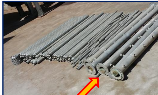
Gypsum accumulation bending steel structure of activated carbon electrolyte filter
