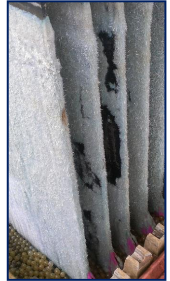
Gypsum crystals formed on Cu EW anodes owing to Ca saturation of electrolyte
