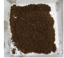
Alkaline Pre-oxidation ( 99% S conversion ) Conditions: 75 °C, 2:1 K:S molar ratio, KOH, 16-24h
