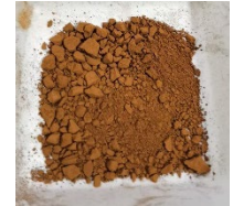
Copper leaching ( 95% Cu extraction ) Conditions: glycine-Cu 4:1 molar ratio 30 °C, pH 10.5-11, 24-30 hours ( GlyLeach™ )
